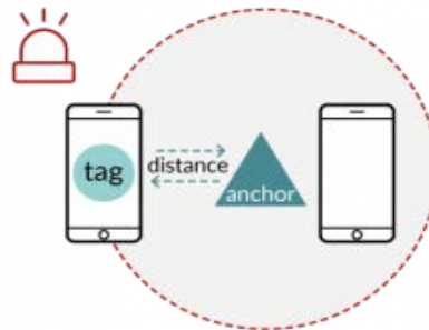
Secure Bubble Point-to-Point Two-Way Ranging (TWR)
